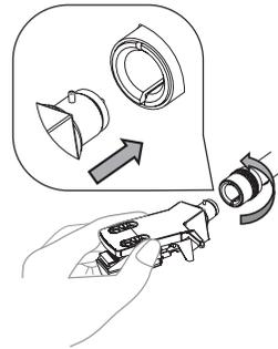
4. Attach the counterweight onto the tonearm.
