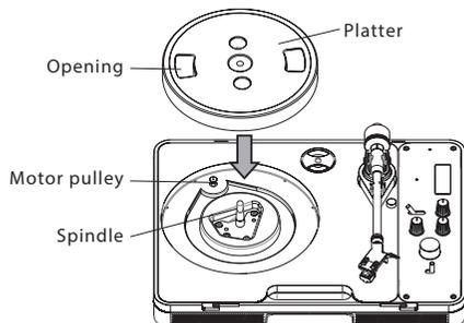
2. Attach the belt to the motor pulley.
