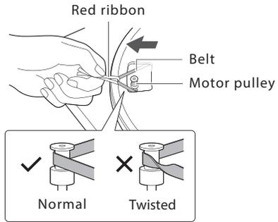
The belt should not be twisted when you attach it to the pulley. Remove the red ribbon.
