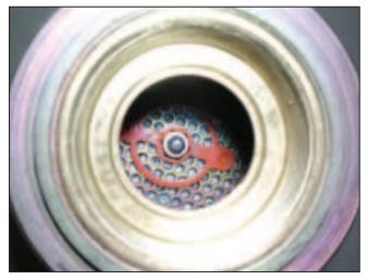
Figure 7. Silencer with a red INTERNAL WEAR indicator.
