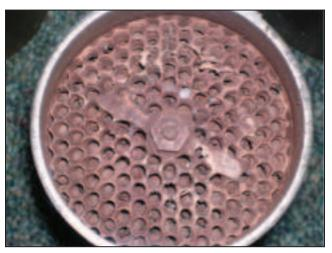
Figure 9. Silencer after three operations at full fault current.
