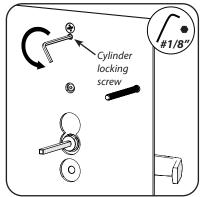
Install cylinder with coil spring and collar into exterior trim by partially inserting key into cylinder and rotating cylinder clockwise into the trim until it bottoms out against the trim back plate. Then rotate counter-clockwise one full rotation to back cam away from back plate.
