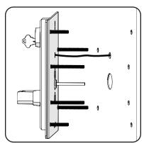
4 Secure trim to mechanism. At the front side of the mechanism, secure trim posts with (2) flat washers, (2) acorn nuts, and (2) K-lock nuts.
