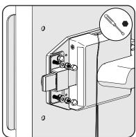
**5** At rear side of mechanism, secure trim posts with (2) acorn nuts and (2) K-lock nuts.
