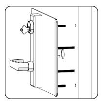
2 If wired, connect the wiring from trim to power transfer.
