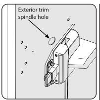
NOTE: Two of the mounting holes for trim are different than previously installed antipry plate. Cover holes on interior using following parts:
