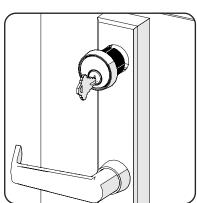
3 Insert hex key (1/8") into cylinder locking screw and rotate clockwise to lock cylinder in place. Jiggle cylinder clockwise/ counter-clockwise to be certain that cylinder locking arms are fully seated into cylinder slots.
