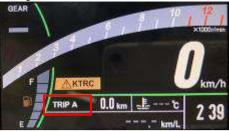
Short press of left button to change the ODO display to TRIP A display , then long press of left and right buttons to enter Menu.
