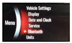
Short press of left button to move the selection to Bluetooth then short press of right button to enter Bluetooth setting.
