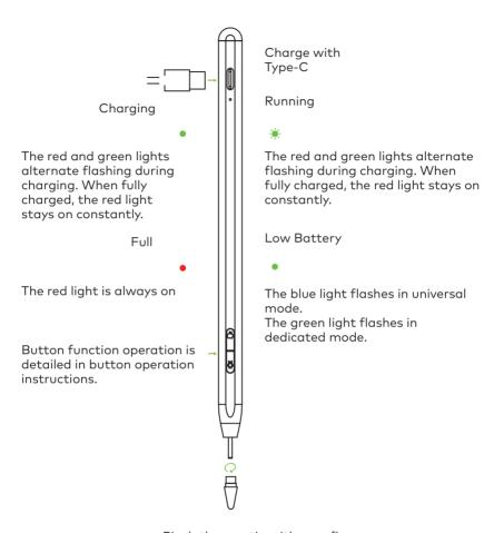
Pinch the pen tip with your fingers, and then rotate the pen tip counter clockwise until it unscrews the pen tube.
