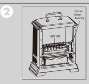
2. Remove back panel to access light bulb.
