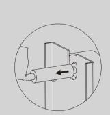
3. Remove the rotation axis in the direction of the arrow.
