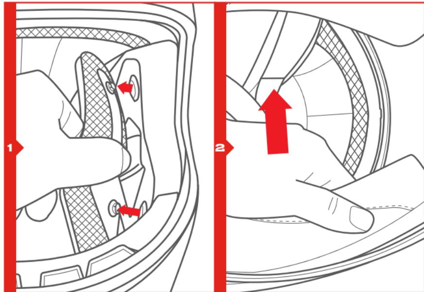
**Installing the side pads**
