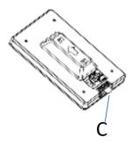
The insulating sheet (C) needs to be removed before use.
