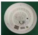
Step 2: Remove the screws from the LED-Board, the Driver and the connection and remove the cable.
