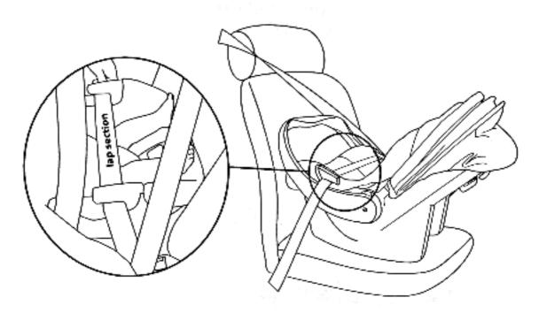
**3.** Pull the diagonal section of the seat belt around the back of the car seat. Place the diagonal section of the seat belt securely into the diagonal belt guide positioned on the back of the car seat. Holding the car seat firmly pull the diagonal section of the seat belt to remove any slack.
