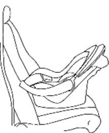
Slowly pull the seat belt out across the car seat and fasten the seat belt. Pass the lap section of the seat belt through both lap belt guides.
