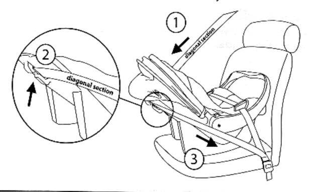
**4.** Fasten the vehicle seat belt. Check that the angle of the car seat back rest is not too upright and make sure the seat belt is not twisted. Push firmly on the back of the car seat. It should feel tight and secure. There should be no excessive movement forward or to the side.
