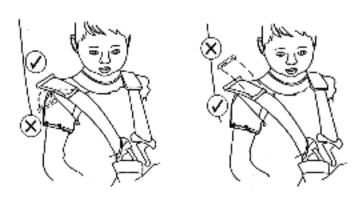
**2.** Position the harness over the baby making sure there are no twists. Fit the shoulder harness fasteners together and then push firmly into the buckle housing. Listen for the 'click'.
