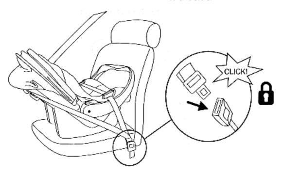
**5.** To remove the car seat from the vehicle, remove the diagonal section of the seat belt from the diagonal belt guide. Unfasten the seat belt and remove the belt from the lap belt guide taking care to hold the seat belt away from the baby.
