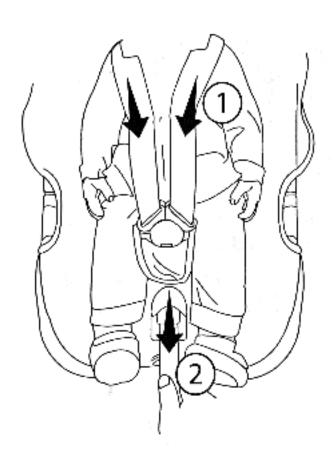
**4.** To remove your child from the car seat, slacken the straps, unfasten the harness and place straps over the side of the car seat.
