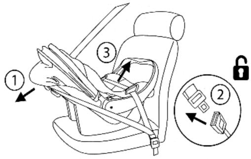
**6.** Adjust the car seat handle to position B and carefully remove the car seat from the vehicle.
