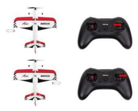
When the aircraft is vertical, toggle the elevator joystick(CH2) to control the aircraft moving forward or backward.
