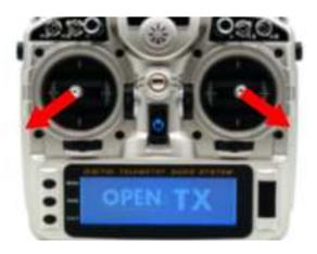
**Note**: When using a non-RadioLink transmitter, if the attitude calibration is unsuccessful when pushing the left stick (left and down) and the right stick (right and down), please change the direction of the channel in the transmitter. Make sure when pushing the joystick as above, the value range of channel 1 to channel 4 is:
