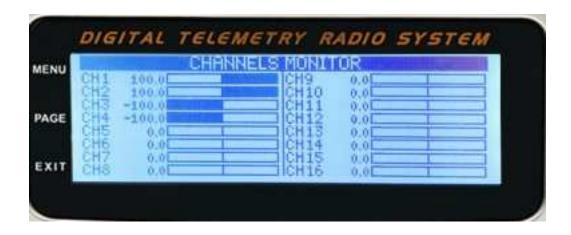
CH1 2000 µs (opentx +100), CH2 2000 µs (opentx +100) CH3 1000 µs (opentx -100), CH4 1000 µs (opentx -100)
