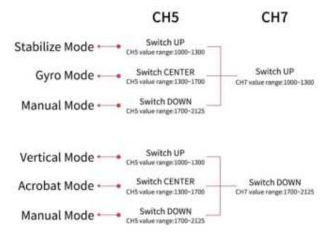
Take AT9S Pro as example. Flight modes are set by CH5(3-way switch SWC) and CH7(2-way switch SWD) as below.
