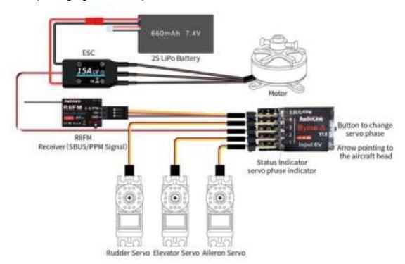
Channels on Byme-A flight controller: CH1-Aileron, CH2-Elevator, CH3-Throttle, CH4-Rudder, S.BUS/PPM-connect to receiver, SBUS/PPM signal supported.
