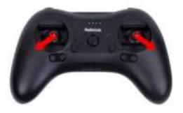
(3) Attitude calibration will be recorded by flight controller once the it is complete with success.
