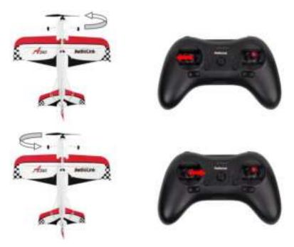
If toggle the throttle joystick(CH3) upward, A560 rises vertically; toggle the throttle joystick downward, A560 descends vertically.
