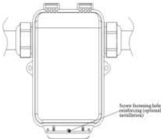
Fig. 4 Fastening screw installation position
