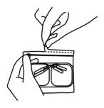
3. Connect one pair of electrode pads to one lead wire and plug the other end of the wire into the A or B output of the device.
