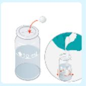
Then, add a Hardicol No2 tablet. Thoroughly crush and stir, until fully dissolved.
