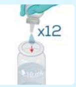
Prepare sample by adding 12 drops of Hardicol liquid buffer and stir.
