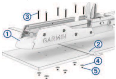
**NOTE:** There are two mounting hole options on the port side of the bow end of the base. You can choose which mounting hole to use depending on the installation angle and the shape of the hull.
