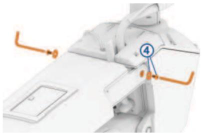
**NOTE:** To properly secure the pin, you should use two hex bits or wrenches so the pin does not rotate as you tighten the screws.
