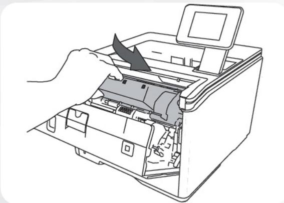
**UK** Place the toner cartridge in the correct position on the printer.
