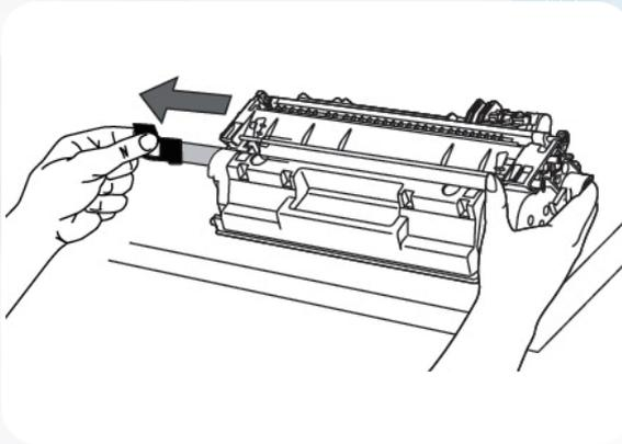
**UK** Place the ink cartridge on a flat desktop and directly pull out the seal.
