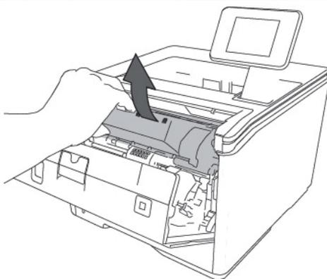
**UK** Pull out the used cartridge from the printer.
