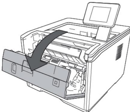
**UK** Switch off the printer and open the front cover.
