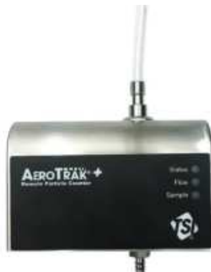
Connecting Sample Tubing to Remote Particle Counter
