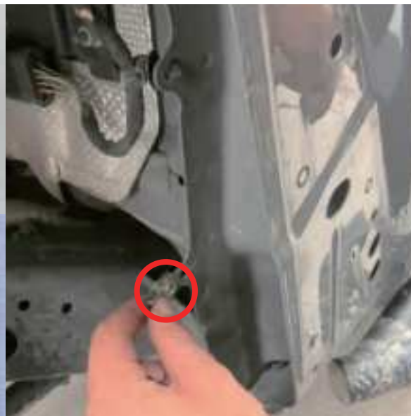
Place the clip nut to the designated holes on the vehicle's body.
