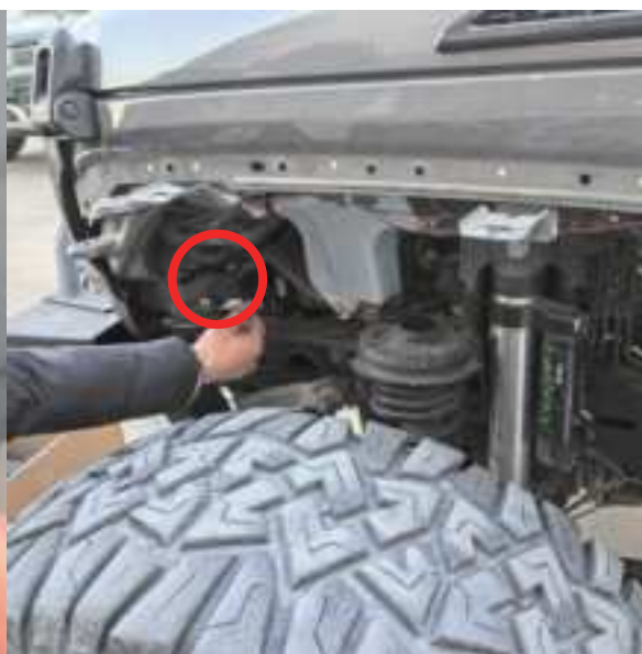
Secure the top mounting point using the bolts, washers, threaded plate (item no.5). Place the clip nut to the threaded plate (item no.5). Note: It is necessary to adjust the bracket to the proper position before tightening the screws.
