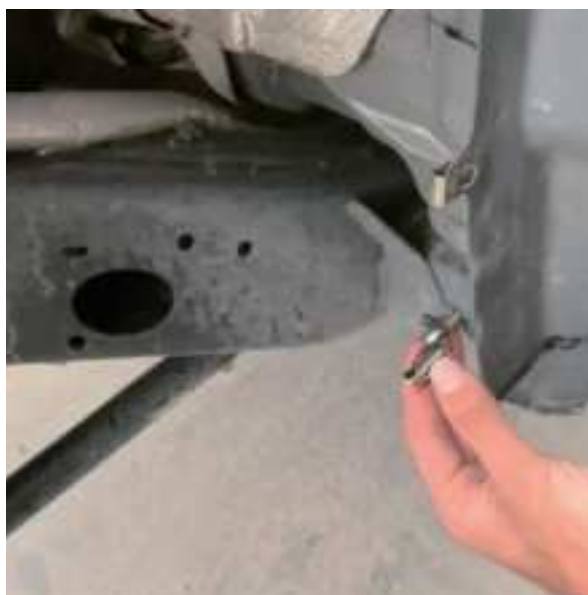
Secure the lower mounting point using the bolts, washers, threaded plate (item no.6). Connected by the clip nut. Note: The U-nut Clip is fastened at the square hole, and the round hole is connected to the vehicle body with a screw.
