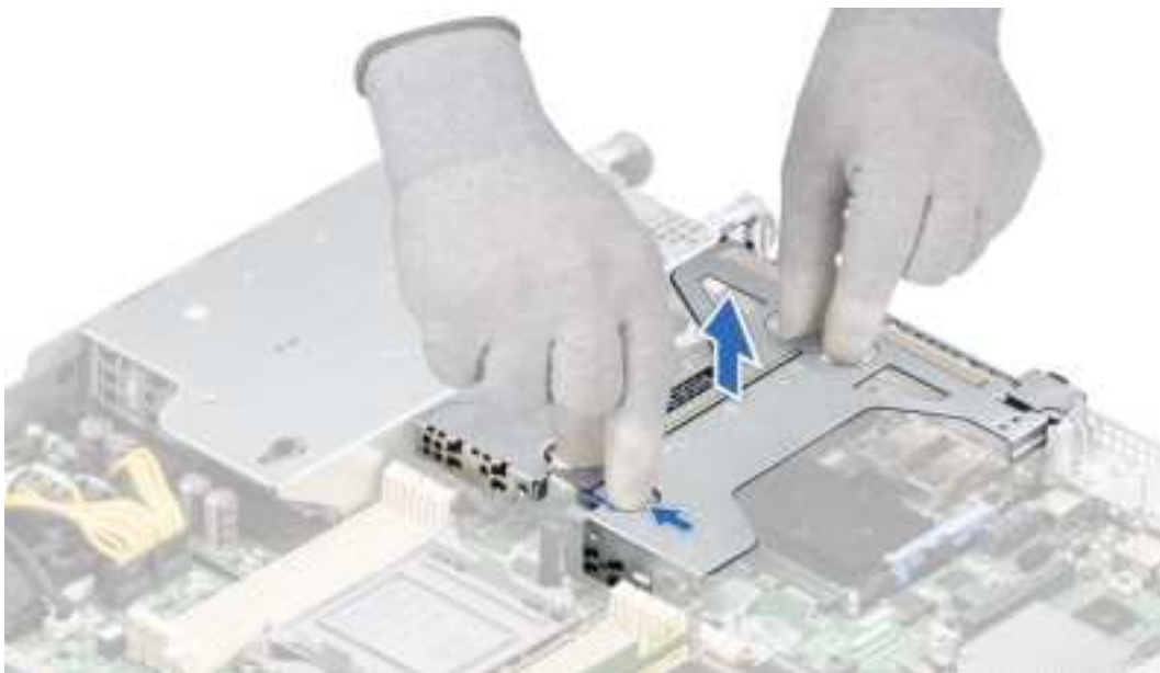
Figure 61. Removing the Riser 2c
