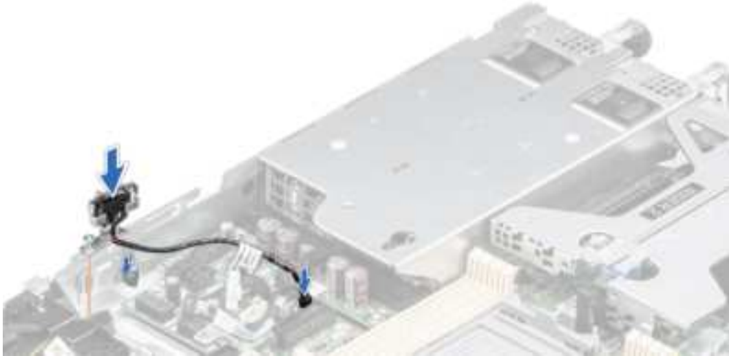
Figure 26. Installing the intrusion switch
