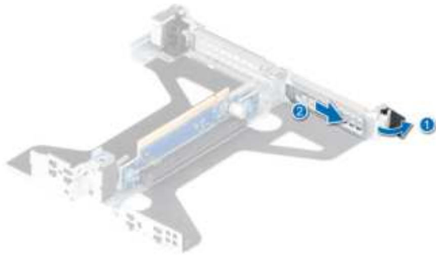
Figure 69. Removing filler bracket in the Riser 2c
