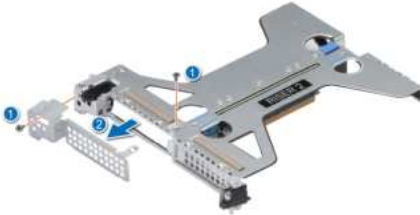
Figure 74. Removing the PCIe blank
