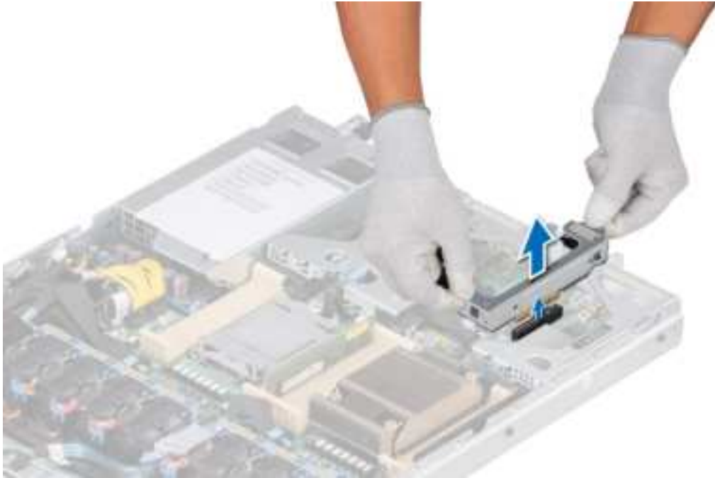
Figure 76. Removing the M.2 BOSS riser
