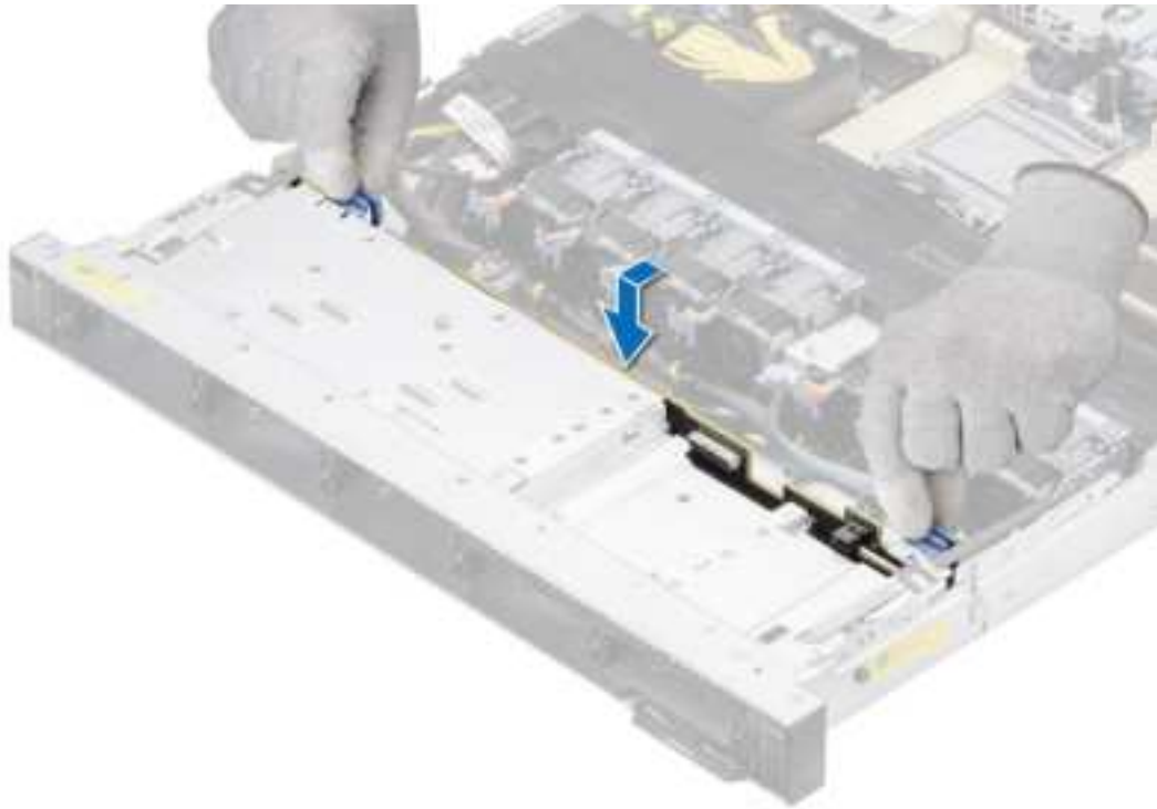
Figure 38. Installing the drive backplane
