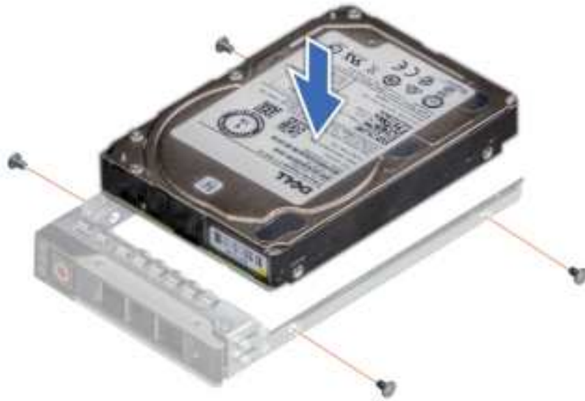
Figure 32. Installing a drive into the drive carrier
