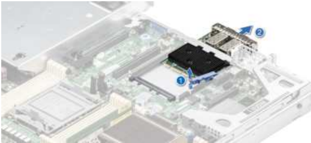
Figure 82. Removing the OCP card
