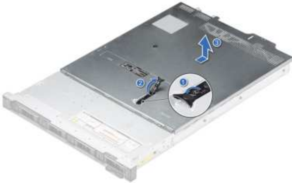
Figure 17. Removing the system cover
