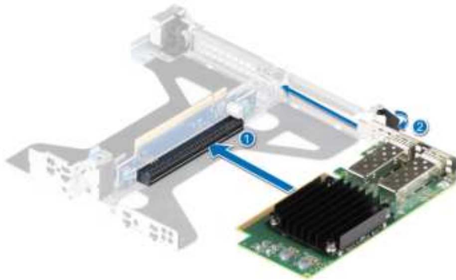
Figure 71. Installing an expansion card into a Riser 2c
