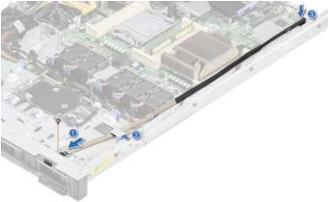
Figure 93. Installing the VGA module
