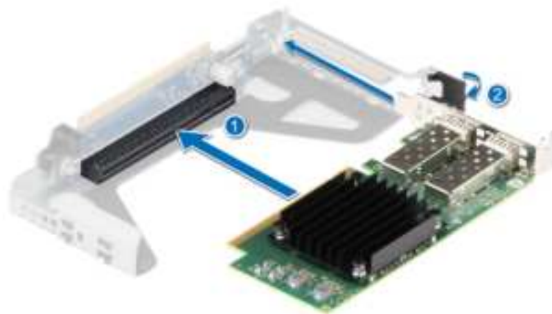
Figure 70. Installing an expansion card into a Riser 1
