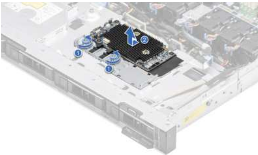
Figure 84. Removing the front mounting front PERC module for 4x3.5-inch system
