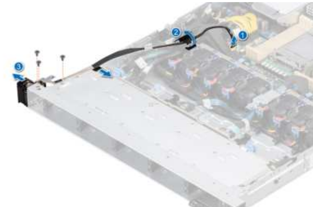
Figure 103. Removing the left control panel
