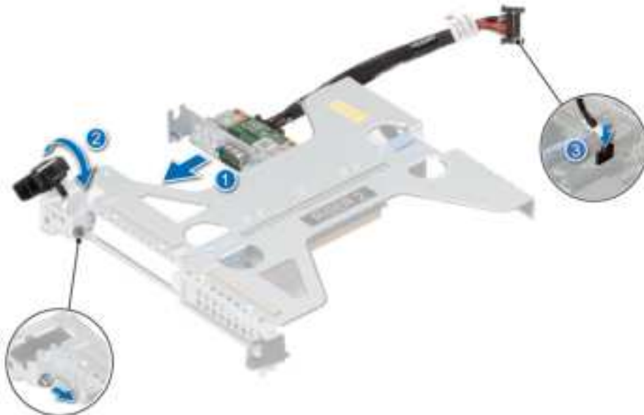
Figure 75. Installing the Serial COM port
