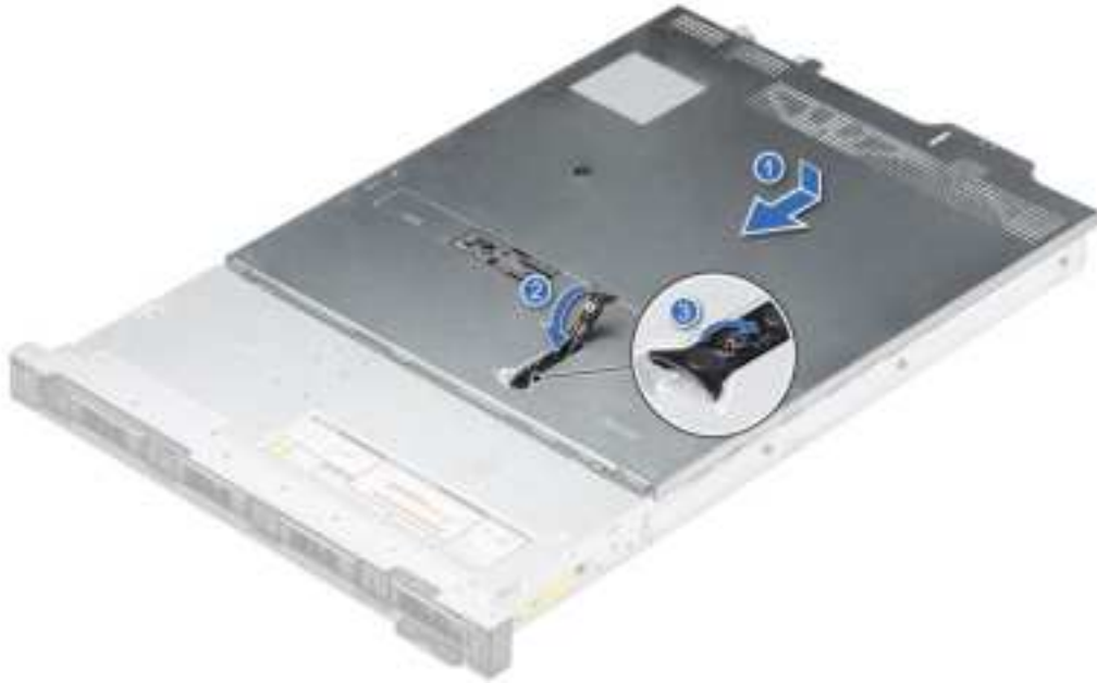
Figure 18. Installing the system cover
