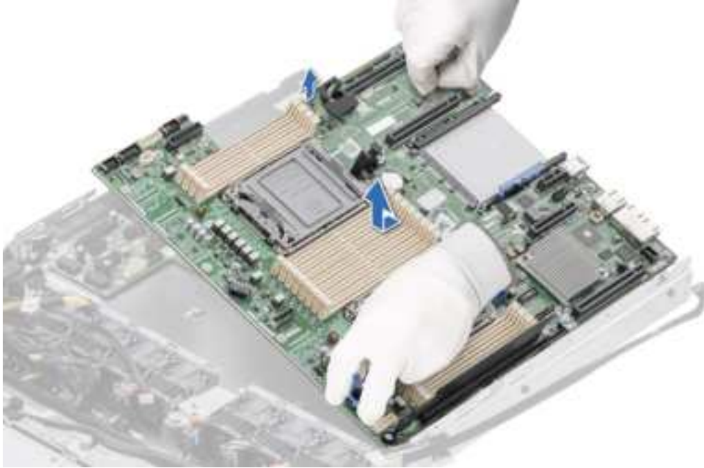
Figure 100. Removing the system board
