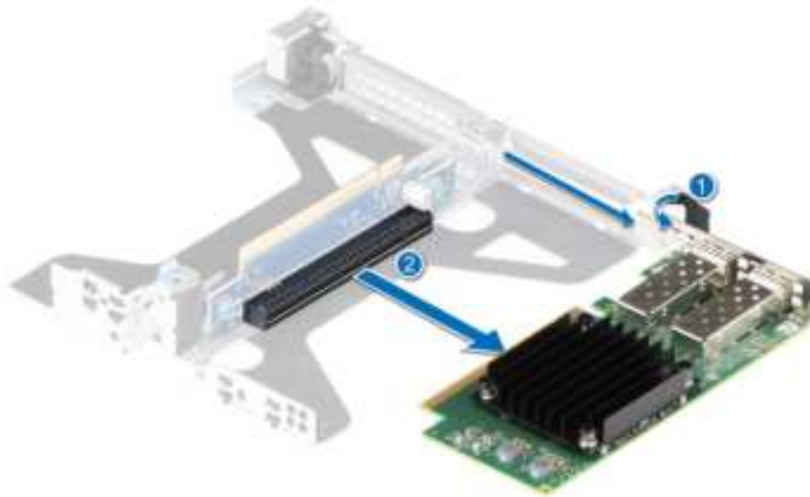
Figure 65. Removing an expansion card from Riser 2c
