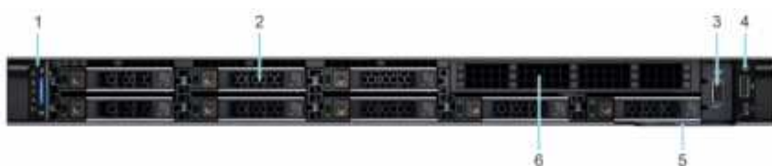
Figure 2. Front view of 8 x 2.5-inch drive system
