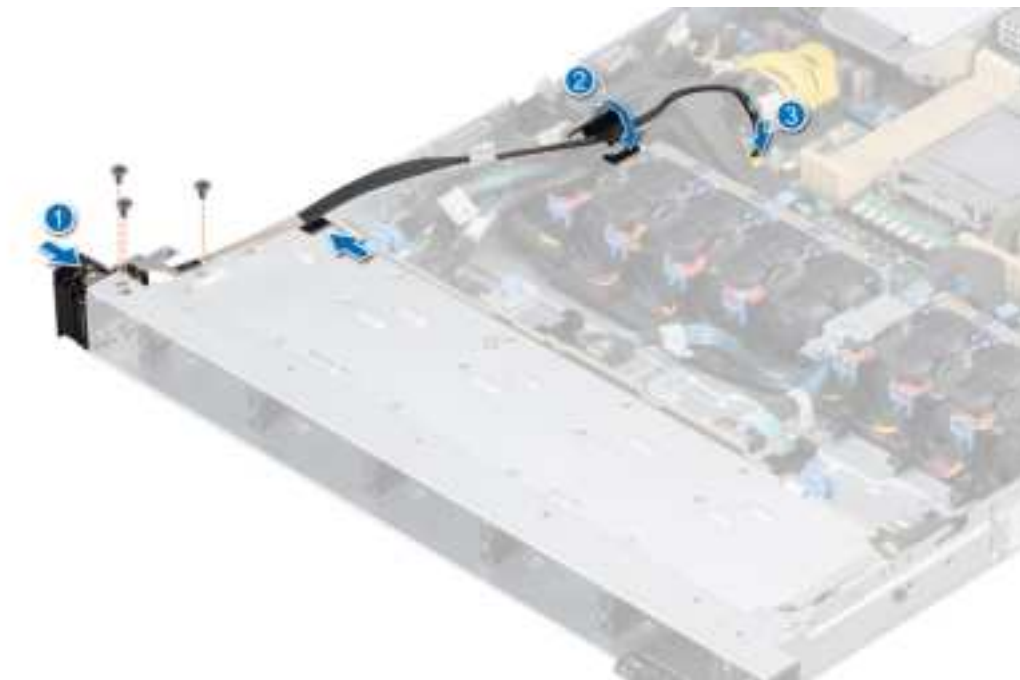
Figure 104. Installing the left control panel
