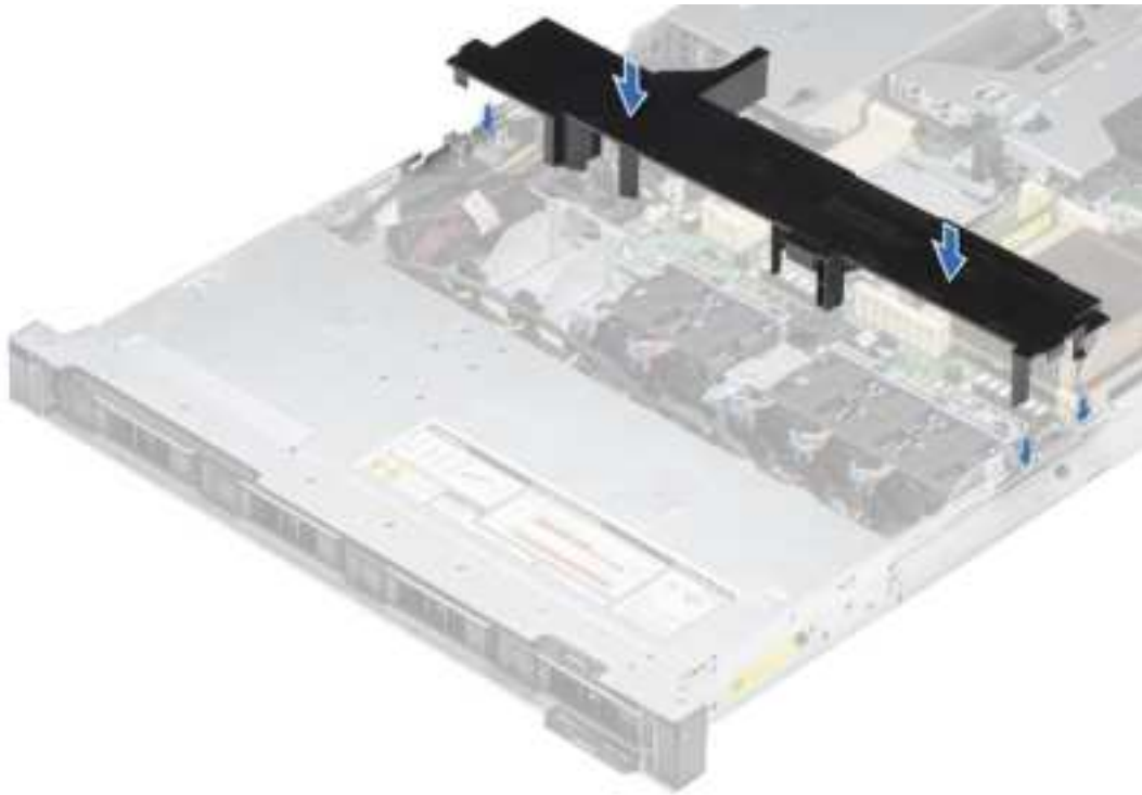
Figure 22. Installing the air shroud
