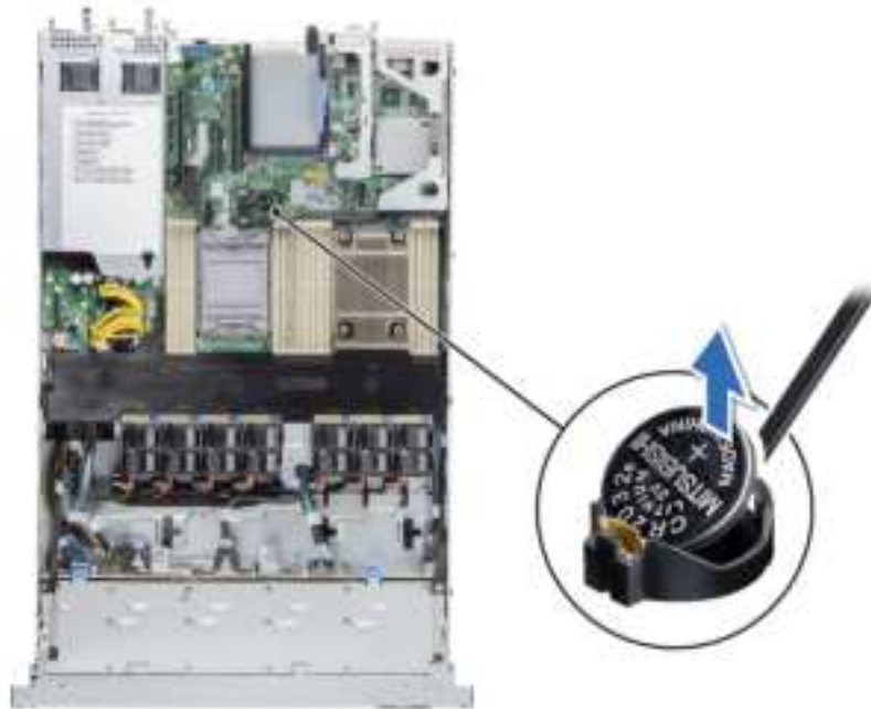
Figure 88. Removing the system battery
