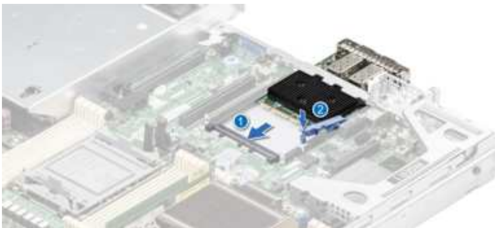
Figure 83. Installing the OCP card
