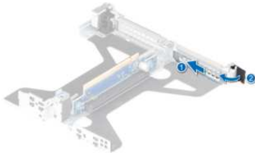
Figure 67. Installing filler bracket in the Riser 2c
