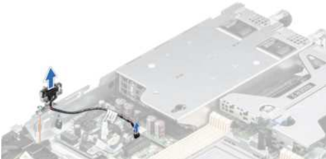
Figure 25. Removing the intrusion switch module
