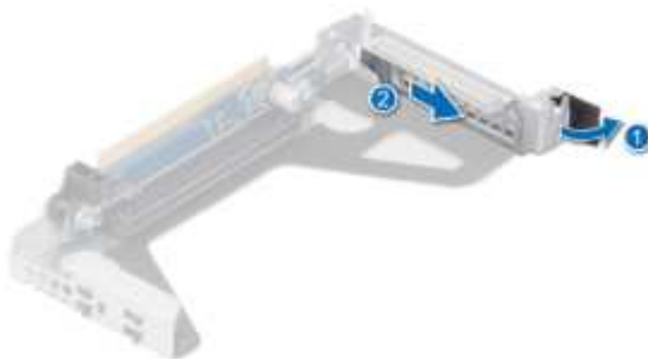
Figure 68. Removing a filler bracket from Riser 1
