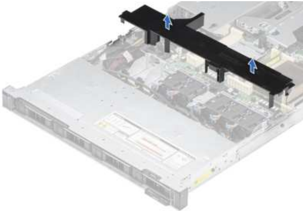
Figure 21. Removing the air shroud
