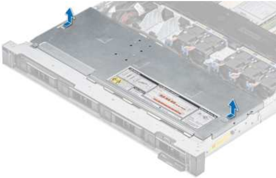
Figure 19. Removing the drive backplane cover
