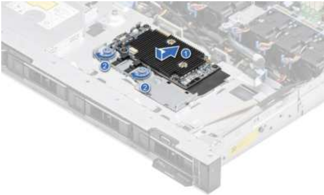
Figure 86. Installing the front mounting front PERC module for 4x3.5-inch system
