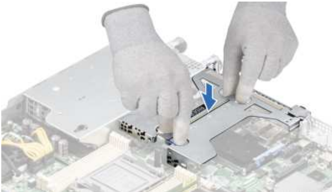
Figure 63. Installing the Riser 2c
