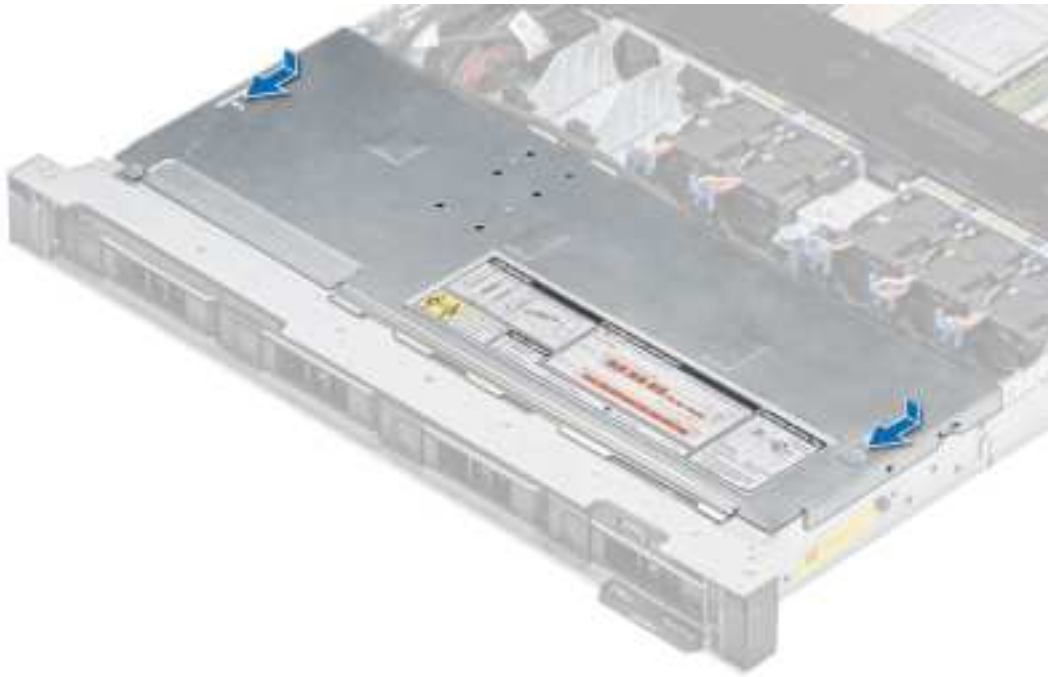
Figure 20. Installing the drive backplane cover
