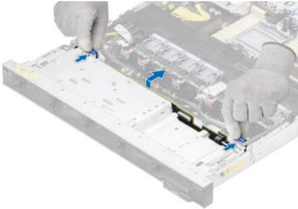
Figure 37. Removing the backplane
