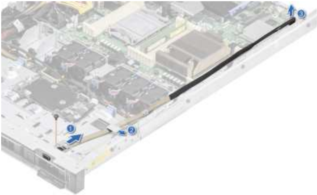
Figure 92. Removing the VGA module
