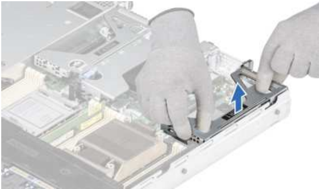
Figure 60. Removing the Riser 1
