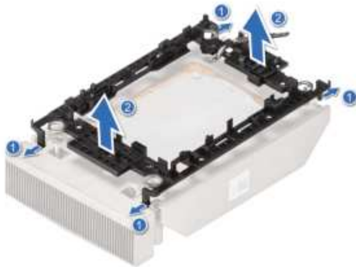
Figure 49. Removing the processor carrier
