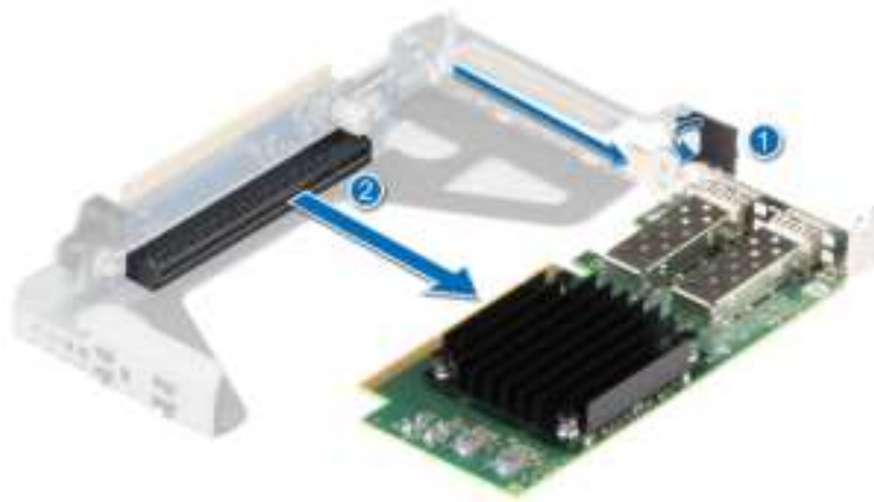
Figure 64. Removing an expansion card from the Riser 1
