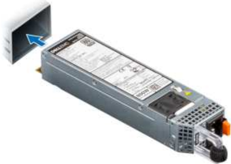
Figure 97. Installing a power supply unit
