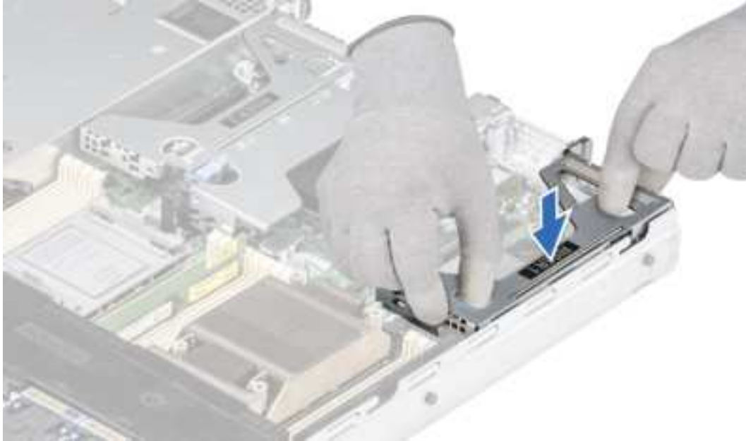
Figure 62. Installing the Riser 1
