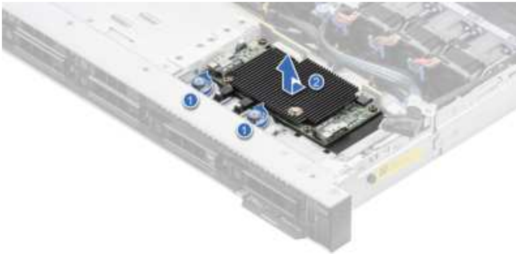
Figure 85. Removing the front mounting front PERC module for 8x2.5-inch system
