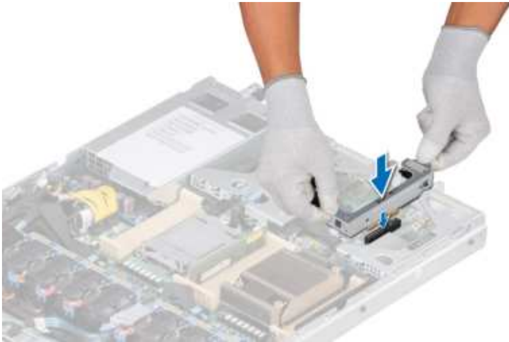
Figure 77. Installing the M.2 boss riser
