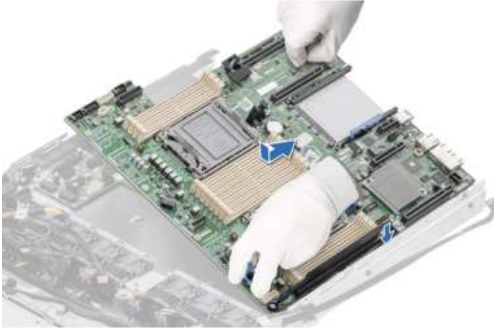
Figure 101. Installing the system board
