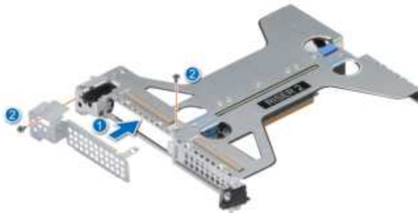
Figure 73. Installing the PCIe blank
