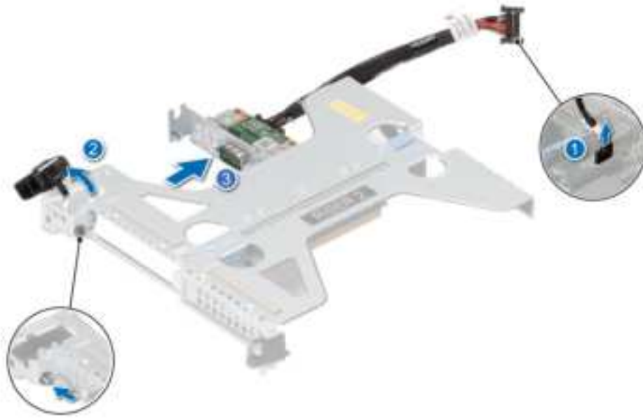
Figure 72. Removing the Serial COM port
