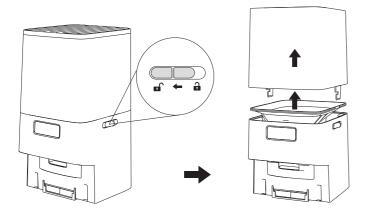
**6** Rotate the four lock latches to unlocked position, then take out the food slider.
