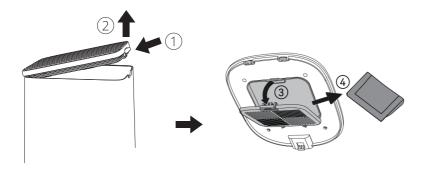
4 Slide the lock latches on both sides to remove the tank and tank base.
