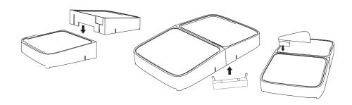
4 The support bars can be installed through the holes at the bottom of the base so as to raise the height.
