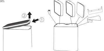
Plug in DC cable. Install 3 x D batteries for back-up power in case of power outage.
