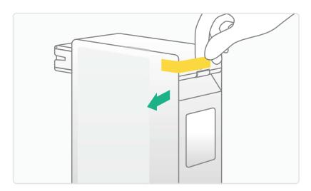
Remove the sticker and open the Material Pod by pulling up on the lid near the handle.
