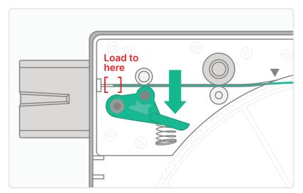
Insert the filament until the tip is in the "Load to here" area. Ensure it is between the two white lines.
