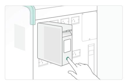
To detach, press the button on the back of the Material Pod. The light will turn green when it is ready to be removed.
