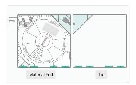
Align the bottom edge of the lid to the magnets on the material pod.
