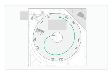
Put the spool into the Material Pod. Ensure that the filament is coming off the spool and towards the drive mechanism in a counter-clockwise direction.
