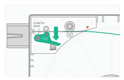
Find the end of the filament and load it into the Material Pod drive system at the spot marked by a triangle (red in the left image). Continue loading while pressing down the green drive arm.
