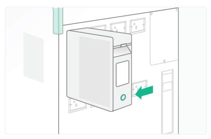
Once detected by Element, the light on the back of the Material Pod will flash green to confirm a successful attachment.
