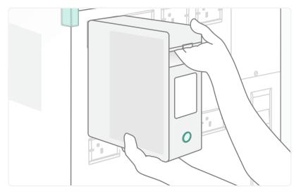
Holding the base of the Material Pod with one hand, use your free hand to press the lever inside the handle to release the Material Pod, sliding backwards from Element.
