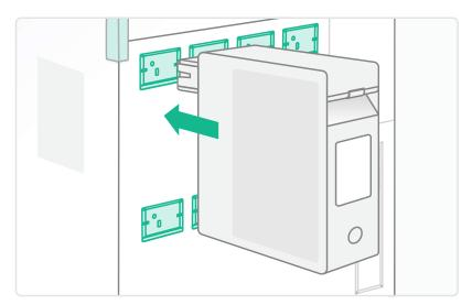
Press the Material Pod outlet into the Element Material Pod receiver until you hear a "click". Use two hands to hold the Material Pod and ensure it is secure before leaving it in place.
