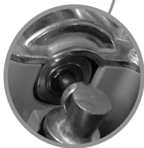
Position of locked motor : the pin should be exited
