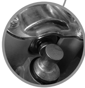
Position of unlocked motor : the pin should be pressed
