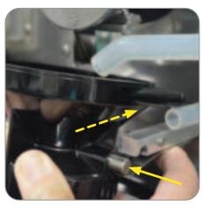
Place the Metal Pins on the Flat Springs.
