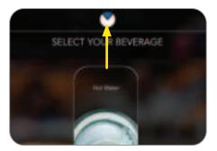
Press and hold the BUNN logo at the top of the screen for 3 seconds to access the Service Access screen.
