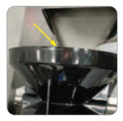
5. To reinstall the funnel, tip the top edge of the funnel under the Coffee Chute.
