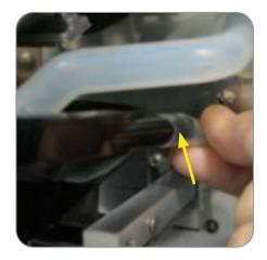
Slide the Rubber Hose (attached to the Brew Funnel) towards the rear of the machine to disconnect it from the Brew Funnel.
