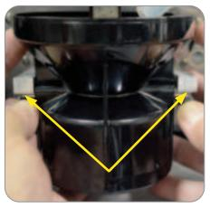
3. While pressing down on both Flat Springs under the funnel arms, pull the funnel down and forward to release it from the funnel arms.
