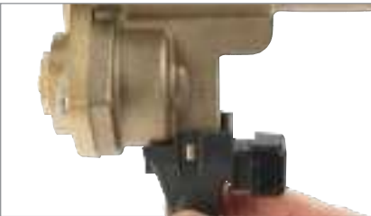
3. Check that the sensor is firmly seated on the relief valve tabs.
