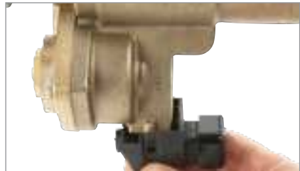
2. Push the sensor onto the relief valve.
