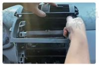
3 Unscrew the four screws on both sides of the original radio, remove the radio, and unplug the wires connected to the original vehicle.
