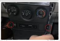
3 Reinstall the decorative side trims on both sides of the radio and the air conditioning control panel back into the original positions in the car. The installation of the new radio is now complete.
