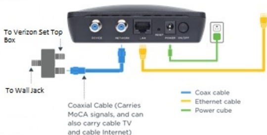
Figure 4. Installing MM1025 with Verizon set top box
