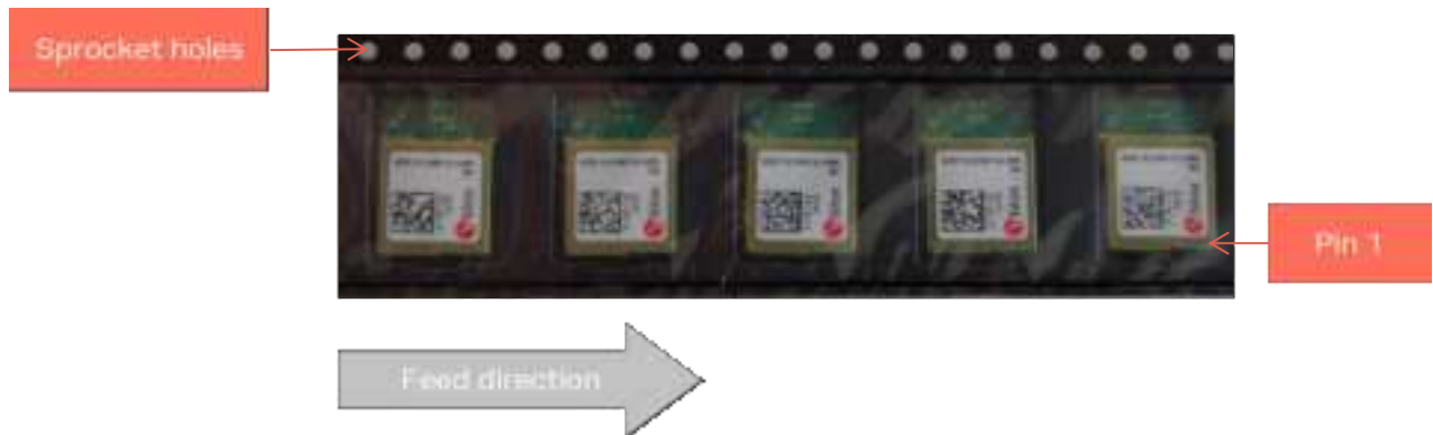
Figure 17: Orientation of MAYA-W4 modules on tape
