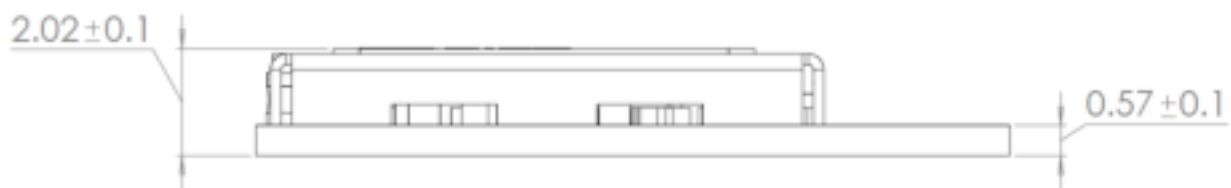
Figure 14: Single pin, dual pin, and internal antenna variants - mechanical specifications (side view)
