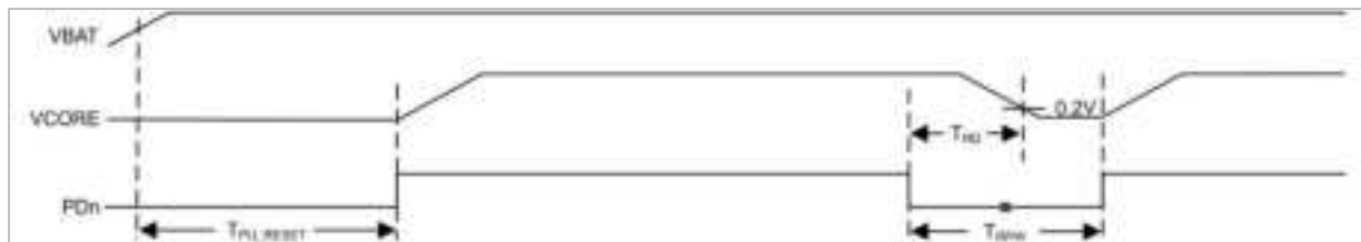
Figure 10: Power-down (PDn) timing
