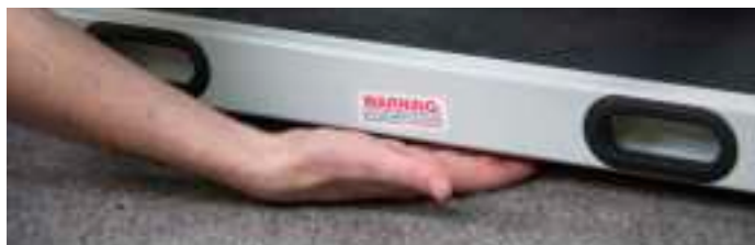
Figure 2-3. Scale Base Clearance
