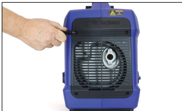
Figure 16 Remove the Muffler Access Cover
