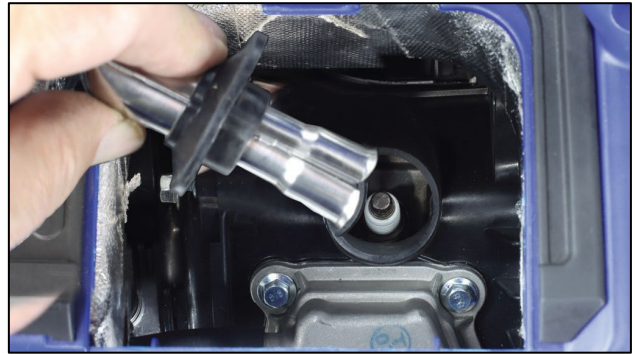
Figure 29 Remove the Spark Plug Boot
