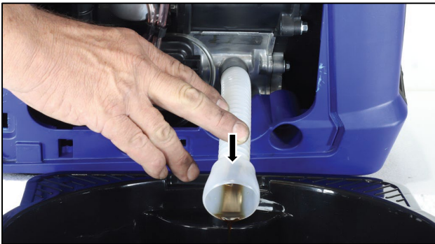
Figure 20 Draining the Engine Oil
