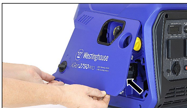
Figure 15 Remove the LHS Access Cover
