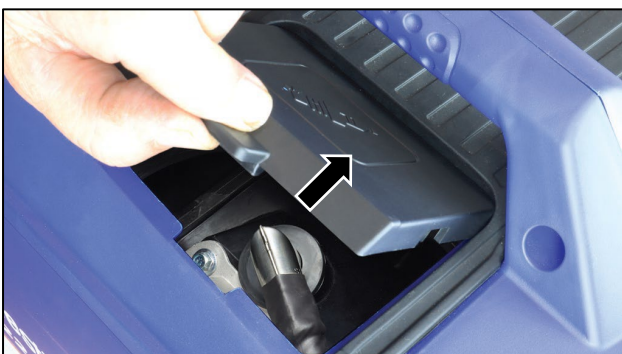
Figure 28 Remove the Spark Plug Access Cover
