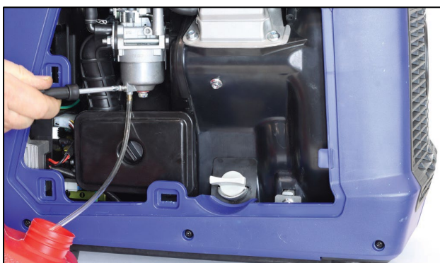
Figure 26 Drain the Carburettor
