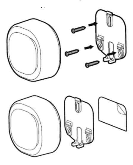
b. Lock the Doorbell 6 into place where the mount is installed.
