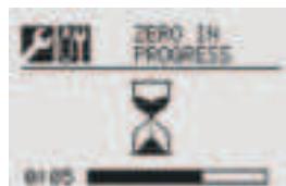
Figure 195. Zero Calibration in Progress
