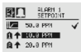
Figure 87. Alarm Limits screen
