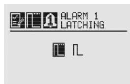
Figure 95. Setting Alarm Latching/Unlatching screen
