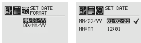
Figure 67. Set Date Format screen / Set Date menu
