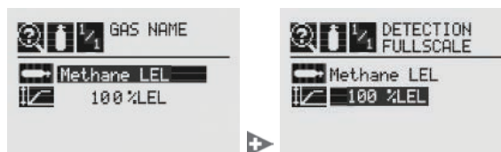
Figure 175. Gas Abbreviation and Full Scale screens
