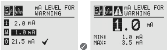
Figure 101. Set mA Levels for Warning screens
