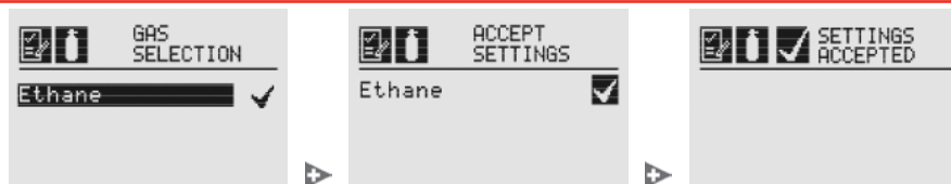
Figure 79. Select New Target Gas screens
