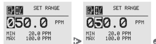
Figure 84. Setting the range value
