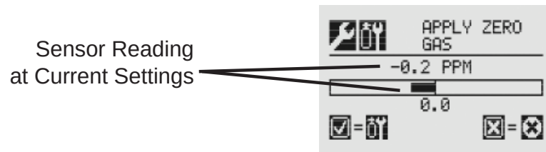
Figure 205. Apply Zero Gas screen
