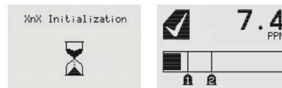
Figure 61. XNX Initialization and General Status screens
