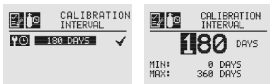
Figure 105. Edit Interval and Setting Interval Value screens
