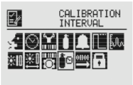
Figure 104. Calibration Interval menu
