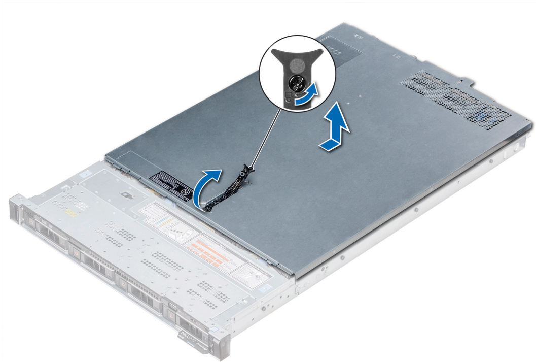
Figure 21. Removing the system cover
