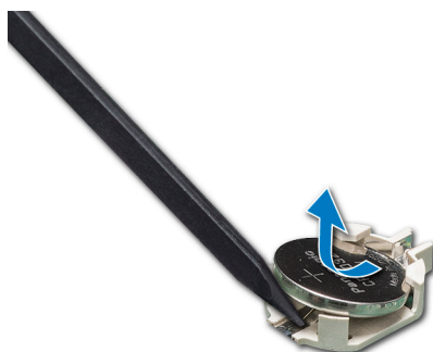
Figure 97. Removing the system battery
