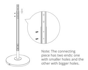
Take the second Pole B, align its metal slots with the bigger holes of the connecting piece, and tighten them with two screws.
