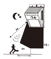
The light will remain ON for 15-25 seconds after no motion is detected.
