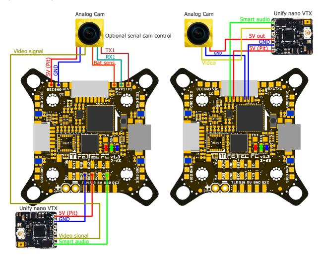
Note: RX and TX connection is only used for cameras which support serial connection
