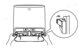
2. Please follow the instructions to place the station against a wall and at a location that is easily accessible, and try to remove obstacles within 1.6ft/0.5m to the left and right of the station and 4.9ft/1.5m to the front. Clean the ground around the station to ensure no oil or water stains.
