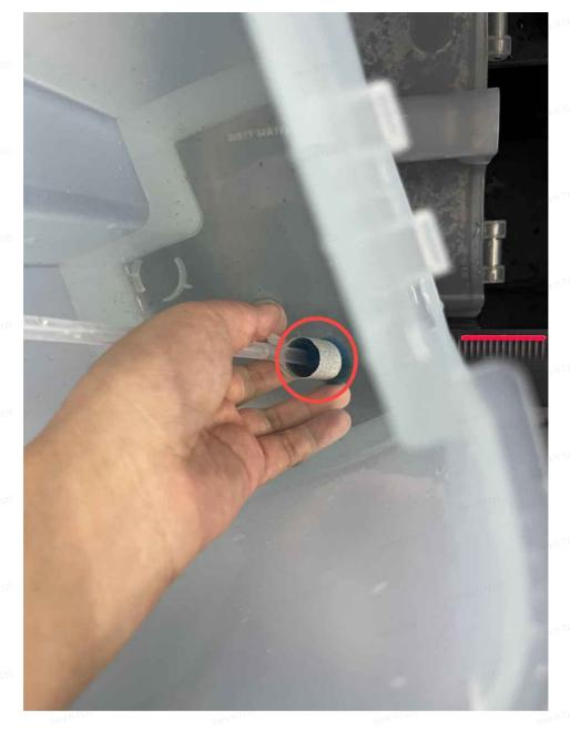
5. Confirm whether the water pipe of the clean water tank is loose. If it is loose, please reconnect the water pipe.
