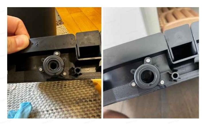
• If you remove the cleaning tray and the water inlet plug is not missing, the cleaning tray may be the cause of water leakage and it needs to be replaced.
