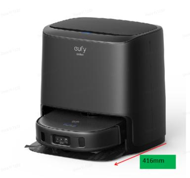
Note: The **station's height** when the **lid is opened** (from the **bottom** of the station **to the lid being opened**) is about **730mm**. When installing the station in the cabinet, it is highly recommended to pay attention to the height mentioned above to ensure you have enough space.
