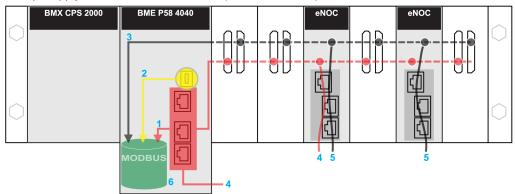
**red:** These requests are sent to the IP address of the CPU. **yellow:** These requests are from the USB port of the CPU.
