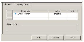
Use the **Check Identity** parameter to set the rules that the CPU's DIO scanner service uses to compare the configured versus the actual remote device:
