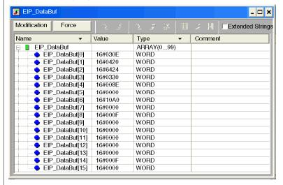
**Note:** Each word presents 2 bytes of data in little endian format, where the least significant byte is stored in the smallest memory address. For example, '0E' in EIP\_DataBuf[0] is the low byte, and '03' is the high byte.
