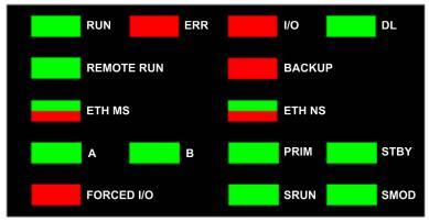
**NOTE:** The **SRUN** and **SMOD** LEDs apply only to safety CPUs.
