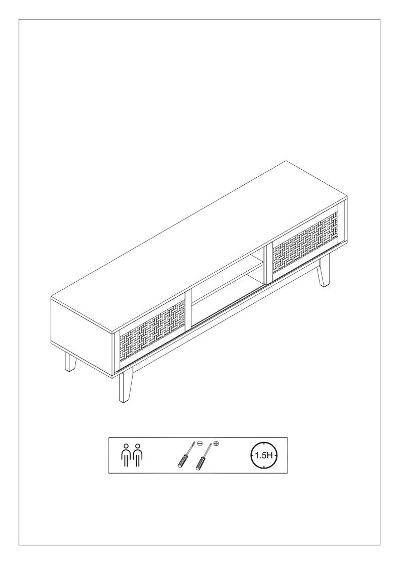
CAUTION: When tightening the screws, tighten sequentially. Do not tighten any screws fully and then towards the next one. When every part is OK, then tighten all the screws.
