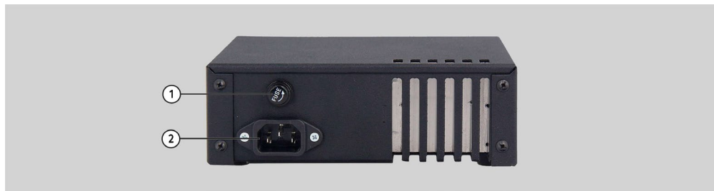
Fig.3. MS021 tester. Back view: 1 – Diode fuse; 2 – Power connector.
