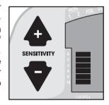
While higher levels of sensitivity enable detection of deeper targets, operation at high levels of sensitivity make the detector **more susceptible to electromagnetic interference**. Higher sensitivity settings can also lead to false signals in difficult ground conditions. Use lower sensitivity settings to suppress interference or false signals from soil minerals when necessary.
