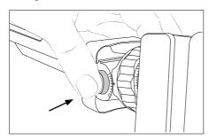
By pressing the button you can rotate the tool holder up or down.
