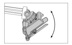
The movement allows a rotation between  $-40^{\circ}$  and  $+40^{\circ}$ .
