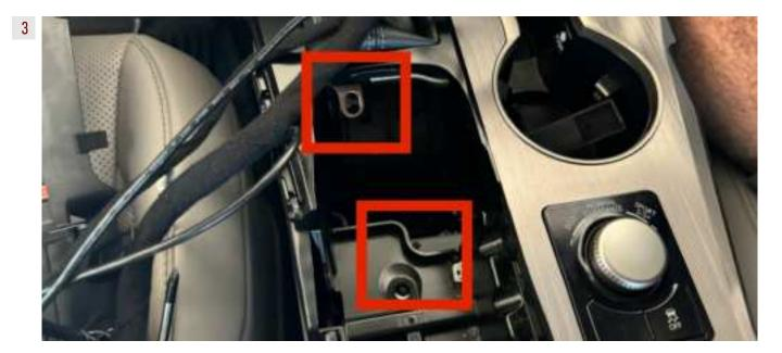
Under where the mouse assembly used to sit, use a Phillips head screwdriver to remove the two highlighted screws.
