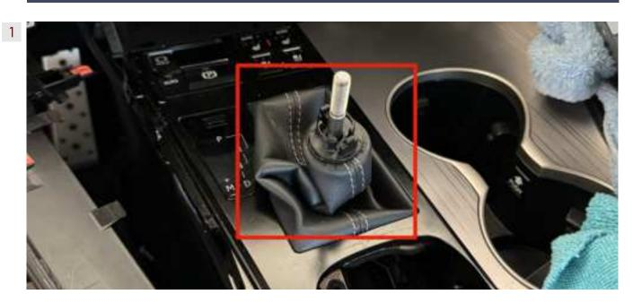
Firmly grip the boot around the shift knob and press it down to separate it from the shift knob. You can now turn the shift knob counter clockwise and thread it off the gear shift stalk.
