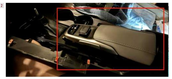
Open the armrest lid. Firmly grab the mouse assembly by the "metal" sides below the leather portion. Rock the mouse assembly side to side with upward pressure and it will come loose. Disconnect it and set it to the side.
