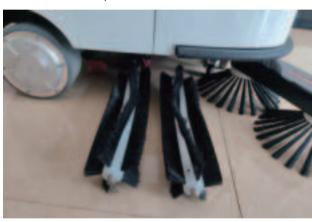
When installing a new roller brush, please insert the end of roller brush with square hole inward into socket of roller brush components, and then, the installation will be completed;
