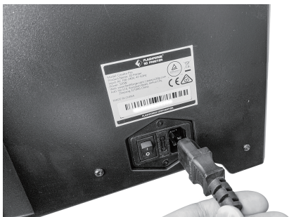
13. Take power cable out and plug it into power input.
