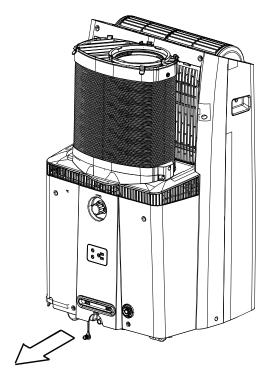
Remove the bottom drain plug to drain the water away.
