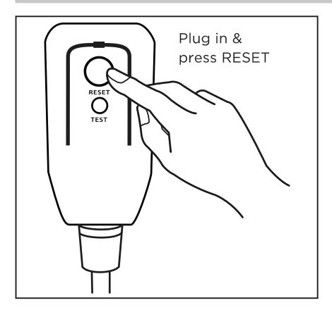
The power supply cord contains a current measuring device that detects damage to the power cord. Test your power supply cord as follows:
