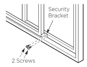
6. If desired, install the security bracket with 2 screws as shown.
