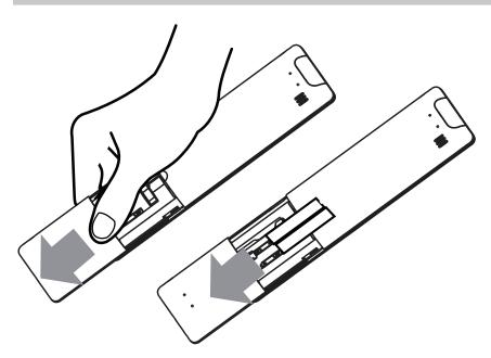
Your air conditioning unit may come with two batteries AAA (some units). Put the batteries in the remote control before use.
