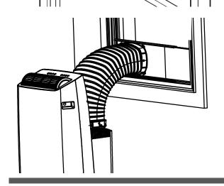
5. Attach the hose to the window slider panel by inserting the end of the hose into the opening on the slider.
