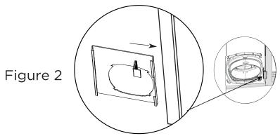
5. Cut the non-adhesive foam seal C strip to match the window height. Insert the foam seal between the glass and the window frame to prevent air and insects from getting into the room.
