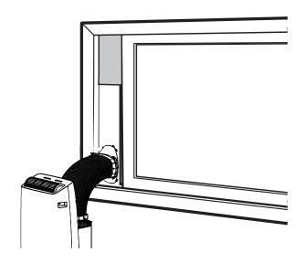
7. Attach the Sliding Window Adapter to the hose by lining up the circles on the adapter.
