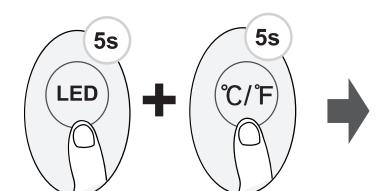
Press together **LED** button and **°C/°F** button at the same time for more than 5 seconds to activate the Lock function.
