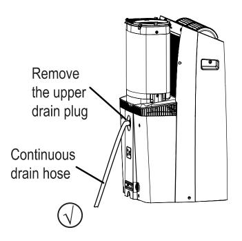
During Dry modes, remove the upper drain plug from the back of the unit and install the drain hose.
