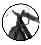
RELEASE FOLDING HINGE TO FOLD STEERING COLUMN
