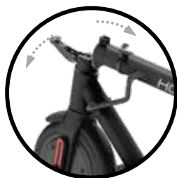
RELEASE FOLDING HINGE TO FOLD STEERING COLUMN
