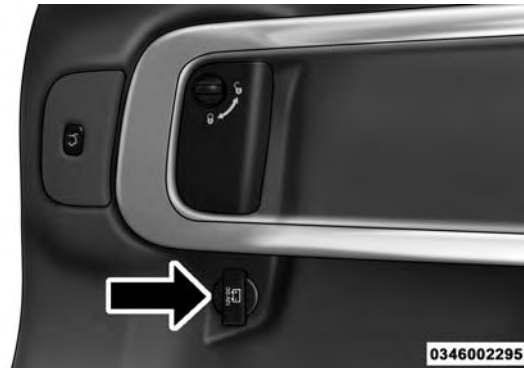
Rear Power Outlet
