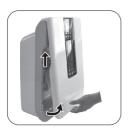
Pull the front plate toward you from its base and its magnets will release the bottom of the front cover. Then lift upward on the front plate to remove it completely, exposing the filter.
